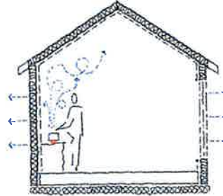
Good insulation to ceiling, walls and floors. vapour-permiable membranes prevent condensation.
